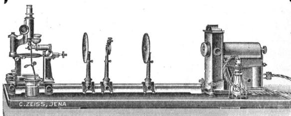
Slit Ultra-microscope for Liquid Colloids
