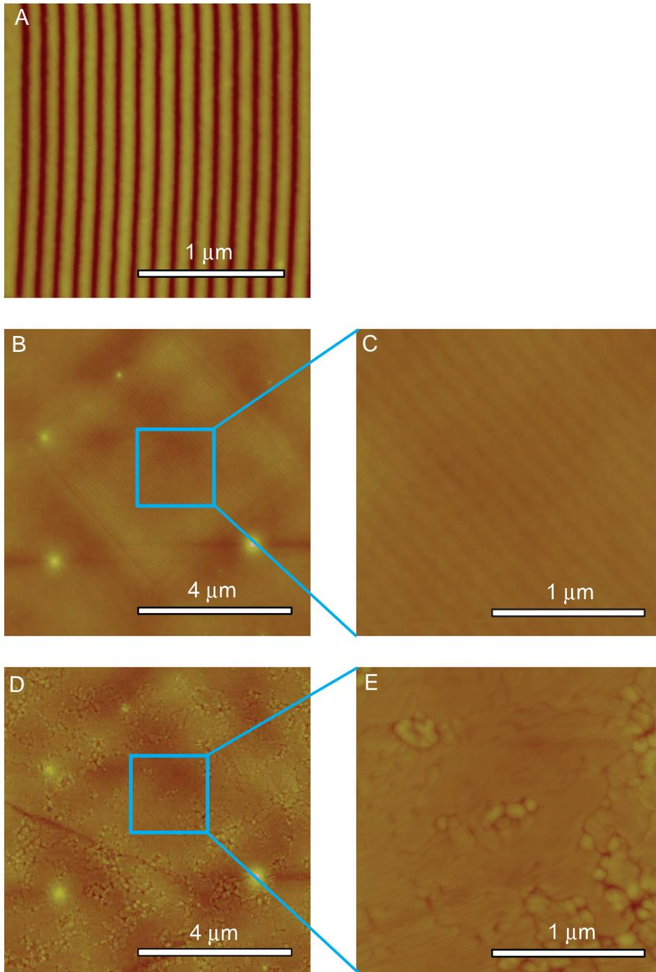
Fig. S2: A. AFM image of the 120nm grating object fabricated using Focused Ion Beam (FIB) lithography into the Cr layer(Fig. S1). B. AFM picture of the surface of planarized PMMA surface and the zoomed-in picture C of the boxed area. The height modulation of the grating object is significantly reduced( $<1.5\text{nm}$ ) by the PMMA layer. D. AFM picture silver superlens
