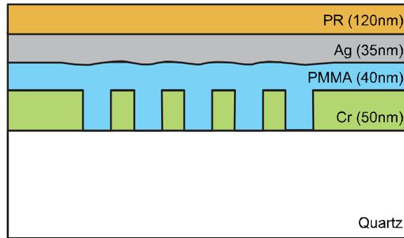
Fig. S1: Sample configuration for superlensing experiment. Cr (50nm) is evaporated on a quartz substrate, and the objects are fabricated using Focused Ion Beam milling. Then, the objects are planarized with a PMMA (40nm) spacer layer and the superlens silver film (35nm) is evaporated onto the PMMA. Finally, near field photolithography is performed to record the image of the sub-wavelength object. Notice the reduced modulation ( $<1.5\text{nm}$ ) on PMMA surface.
