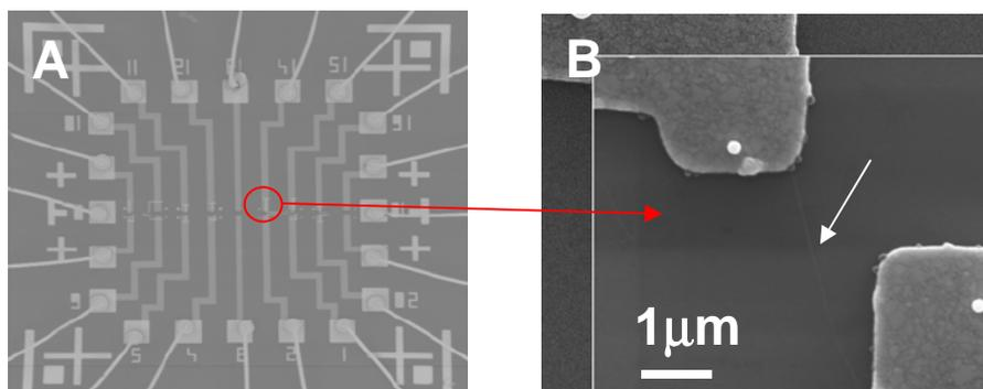
**Fig. S4. Device fabrication and electrical characterization.** (A) and (B) SEM images of the identification marks and contacts. In (B) the arrow indicates the position of the SWCNT incorporated in the device.
