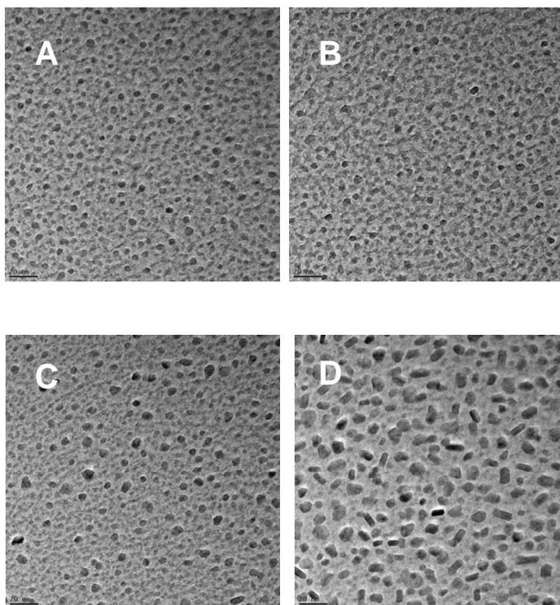
**Fig. S6.** In situ TEM micrographs of Fe catalyst size distribution evolution at 500 °C for 15 min depending on ambient Ar/H<sub>2</sub>O pressure for (A) 1.5 mTorr, (B) 22 mTorr, (C) 550 mTorr and (D) 1200 mTorr. Scale bar is 20 nm.
