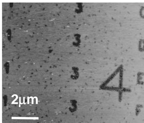
**Fig. S3** The marks on the substrate for identification of individual SWCNTs.
