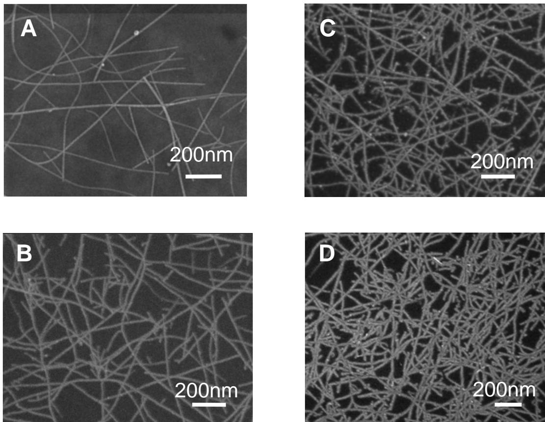
**Fig. S1.** Scanning electron microscope images of SWCNTs on silicon substrate grown from Fe particles preliminarily annealed in: (A) Ar:H<sub>2</sub> (9:1) ambient and (B) Ar:H<sub>2</sub> (8:2) (C) He:H<sub>2</sub> (9:1) and (D) He:H<sub>2</sub> (8:2) ambient in the presence of H<sub>2</sub>O at 860 °C.
