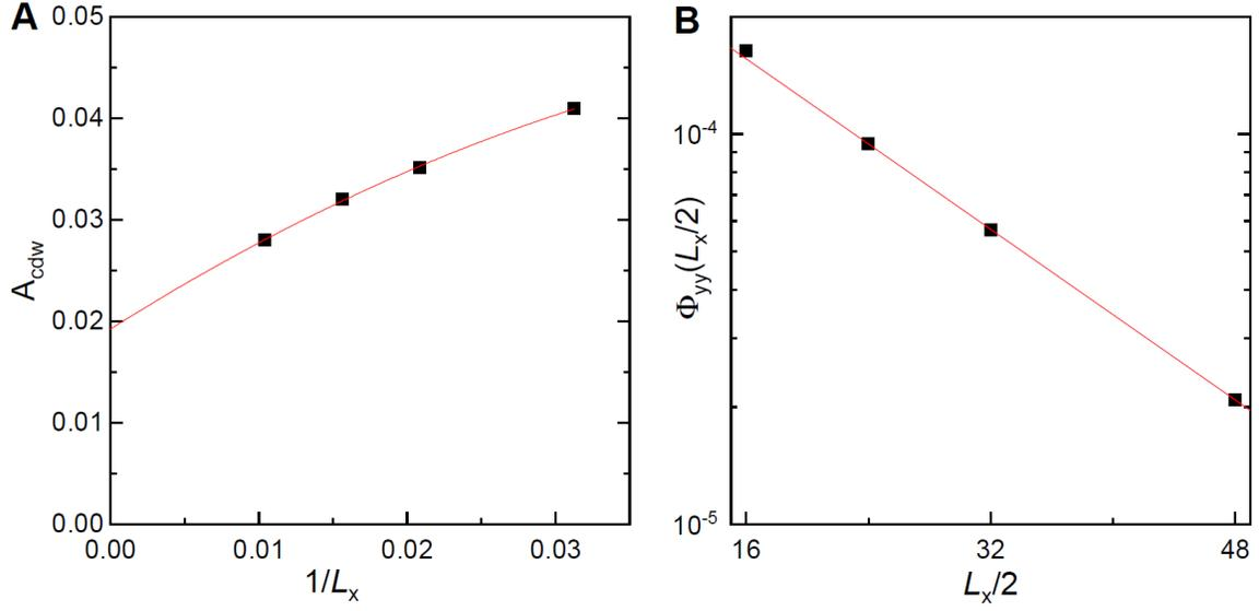
**Fig. S5. The CDW and SC correlations in the filled stripe phase.** Finite-size scaling of (A) the CDW amplitude  $A_{cdw}(L_x)$  in double-linear scale and (B) the SC correlation function  $\Phi_{yy}(L_x/2)$  in semi-logarithmic scale of the  $t$ - $t'$ - $J$  model at doping level  $\delta=12.5\%$  with  $t = 3J$  and  $t' = J/4$  with filled charge stripe ground state. The red line in (A) is the fit using second-order polynomial function and in (B) is the fit using exponential function.
