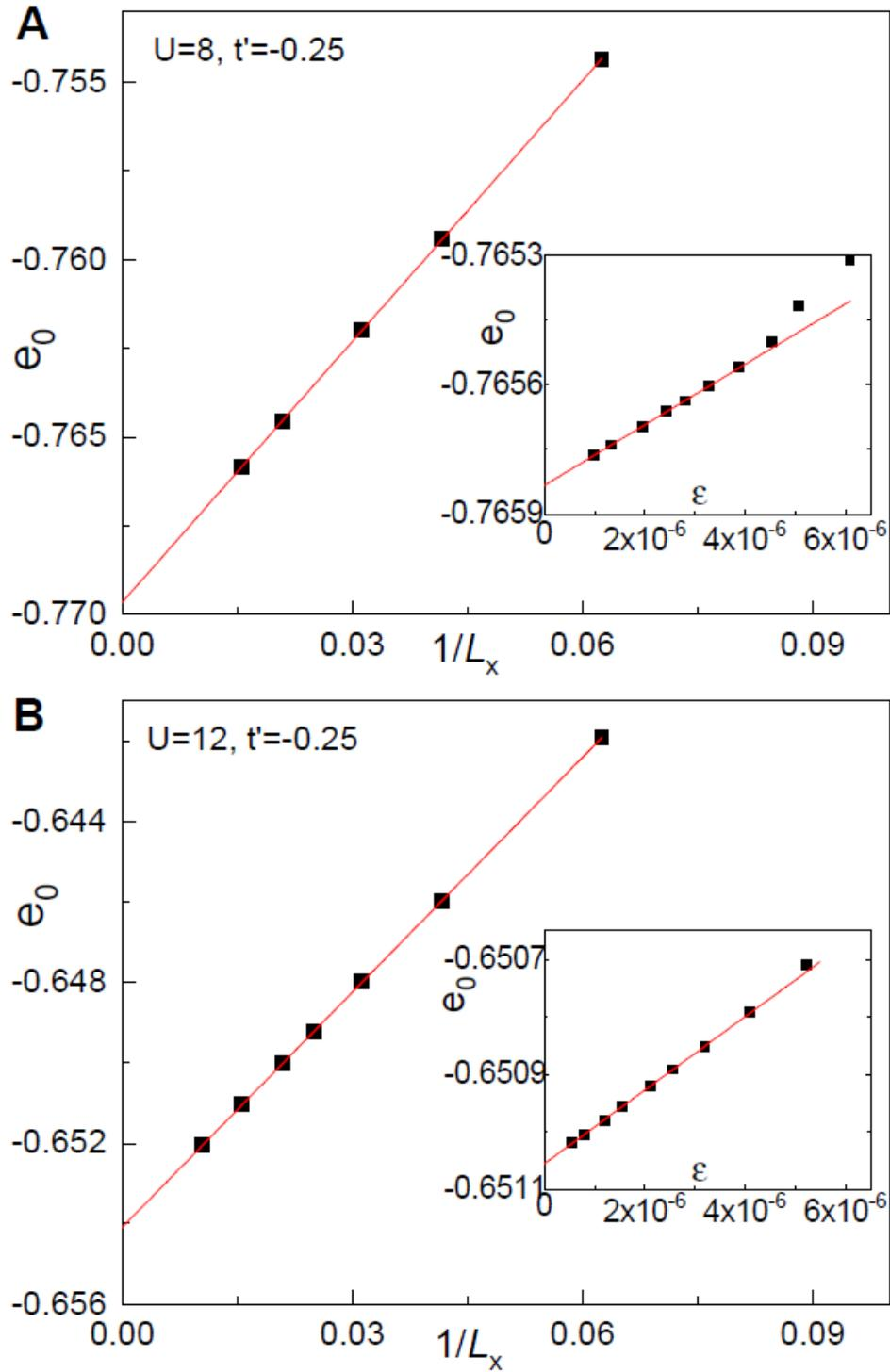
**Fig. S2. Ground state energy of the Hubbard model.** Ground state energy per site  $e_0$  for  $\delta=12.5\%$  as a function of the inverse cylinder length  $L_x$  for (A)  $U=8$  and (B)  $U=12$ . Insets: Examples of truncation error  $\epsilon$  extrapolation of  $e_0$  for  $L_x=64$  cylinders at doping level  $\delta=12.5\%$  for (A)  $U=8$  and (B)  $U=12$ . The red lines show the extrapolation using a linear function.
