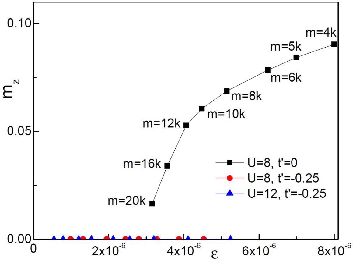
**Fig. S1. Numerical convergence of Hubbard model.** Magnetic moment  $m_z = \frac{1}{N} \sum_{i=1}^N |\langle S_i^z \rangle|$  as a function of number of states  $m$  or truncation error  $\epsilon$  of the Hubbard model at doping level  $\delta=12.5\%$  on  $L_x=64$  cylinders for  $t'=0$  and  $U=8$  (black squares),  $t'=-0.25$  and  $U=8$  (red circles) and  $U=12$  (blue triangles).
