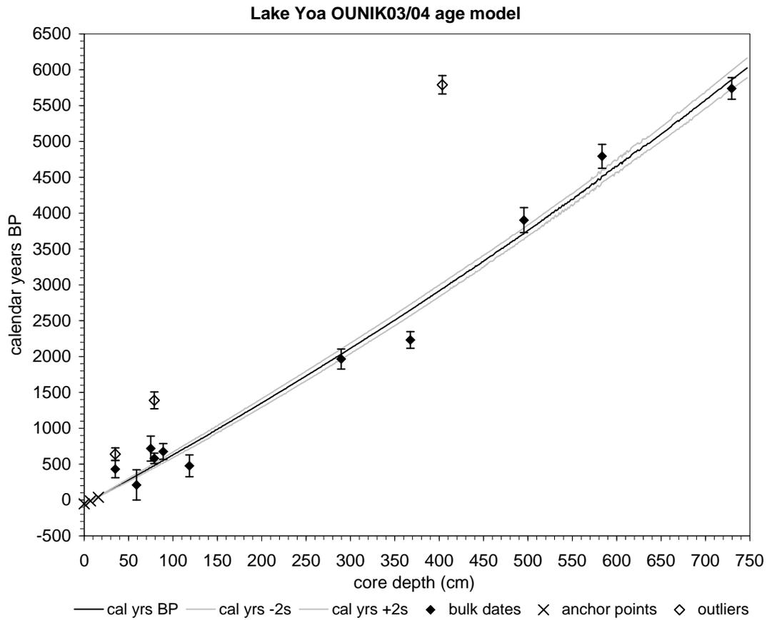
**Fig. S1.** Age-depth relationship of composite core OUNIK03/04 from Lake Yoa, based on a 3rd-order polynomial regression of 3 anchor points and 12 INTCAL04-calibrated  $^{14}\text{C}$  ages vs. cumulative dry weight down-core; see Methods section 2.
