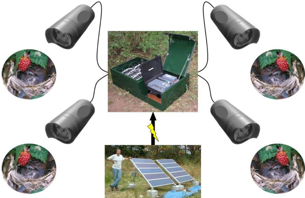
**Fig. S2.** Schematic illustration of one of the custom-built, solar-powered, continuous video surveillance systems used to monitor nests. Each system can record the activity at up to eight nests at a time using miniature, colour/infrared cameras, any of which may be located up to 300 m from the digital recording device (grey unit in green box).
