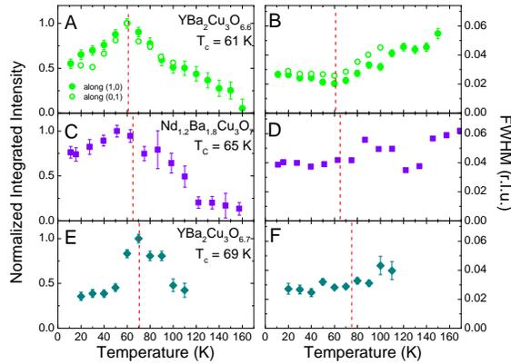
Figure S3: Temperature dependence of the CDW signal intensity and full-width-at-half-maximum (FWHM) in underdoped  $\text{YBa}_2\text{Cu}_3\text{O}_{6.6}$  (A, B),  $\text{Nd}_{1.2}\text{Ba}_{1.8}\text{Cu}_3\text{O}_7$  (C, D), and  $\text{YBa}_2\text{Cu}_3\text{O}_{6.7}$  (E, F), measured using energy integrated RXS.
