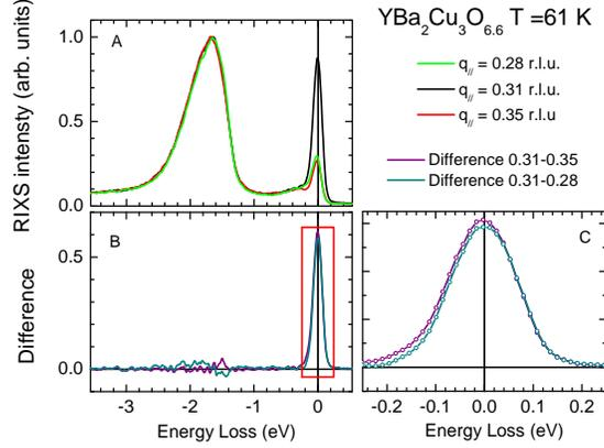
Figure S2: A) RIXS intensity at  $q_{//}=0.28, 0.31$  and  $0.35$  r.l.u. for the  $\text{YBa}_2\text{Cu}_3\text{O}_{6.6}$  sample at  $T \simeq T_c$ . B) Difference between the spectra measured at  $q_{//} = 0.31$  and  $0.28$  r.l.u., and  $q_{//} = 0.31$  and  $0.35$  r.l.u.. C) Low energy enhancement of the panel B.
